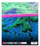
Overlay images of EDX (elemental identification) results on top of SEM image
